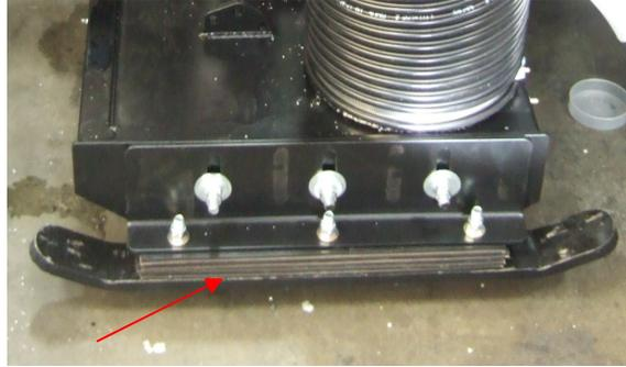
Fig. 17 – Pick-Up Head Skid Spacers.
