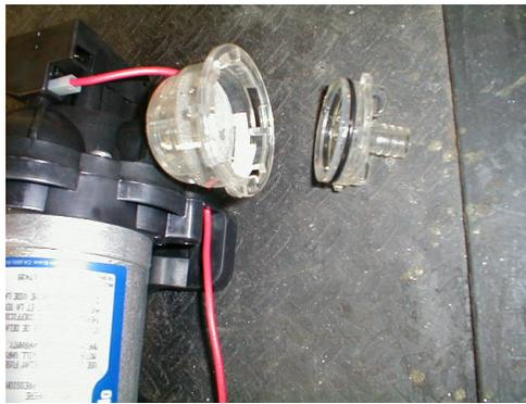
Fig. 26 – Cleaning the Dust Suppression System Water Pump Strainer.
