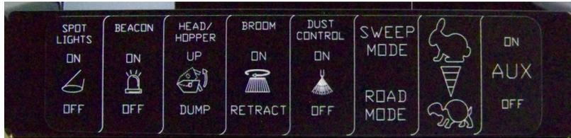
Fig. 3 – Inside view of Conventional Cab with Sweeper Control Panel (Broom model).
