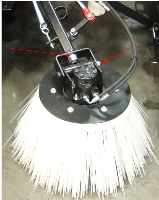
Fig. 10 – Adjusting broom tilt and Pitch.
