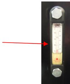
Fig. 31 – Hydraulic Fluid Sight Gauge.
