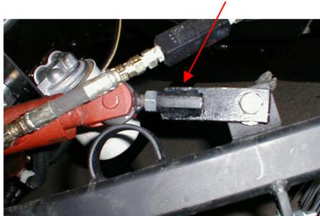
Fig. 11 – Curb Broom Turnbuckle.
