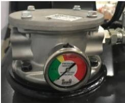
2. Return Filter – the gauge will indicate to the red if filter is clogged and being bypassed. Also check fluid quality in gauge free of contaminants
