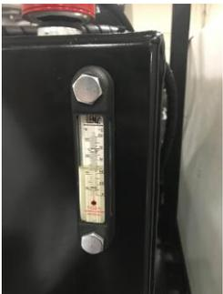
3. Sight Gauge (Reservoir) – if you can not see fluid in this gauge, inspect system for leaks and don't operate sweeper until fluid level is half way up the gauge. Also check fluid quality – free of contaminants
