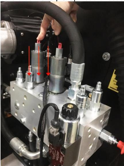
*Hopper Manual Override – Use a small screwdriver*
