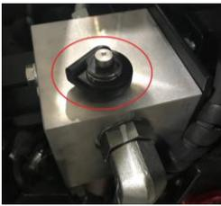
1. Pressure Filter – the clear disc on top will turn red if the filter is clogged and being bypassed
