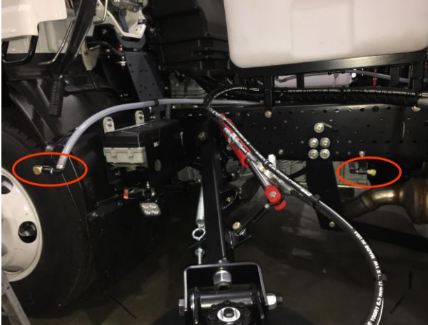
Water System Nozzles (5 Front Spray Bar, 1 Curb Broom, 1 Driver Side Sweeping Head, 1 Passenger Side Sweeping Head)
