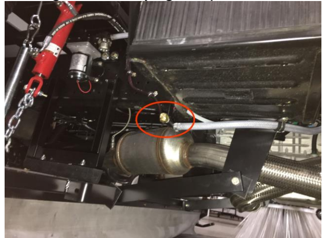
Water System Nozzles (5 Front Spray Bar, 1 Curb Broom, 1 Driver Side Sweeping Head, 1 Passenger Side Sweeping Head)
